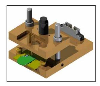
This fixture is easily adaptable to any shape circuit board and pad configuration. Ball bearing bushings and spring loaded pins ensure smooth movement and consistent pin-to-pad contact. These fixtures are efficient, durable, and easy to use.
